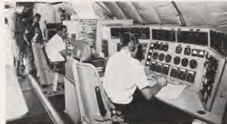
The heart of the automatic system is an elaborate console which monitors navaids.
