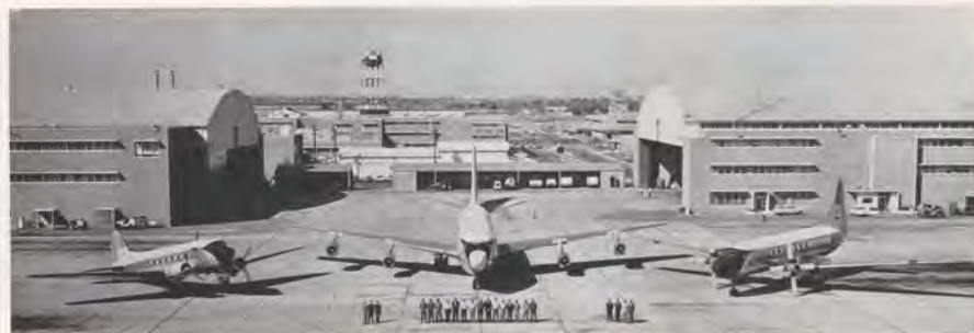
The 'Big Three' and their crews. The DC-3 at left, the C-135 in the center, and the Convair 440 are the three types of FAA aircraft used in flight inspection.
