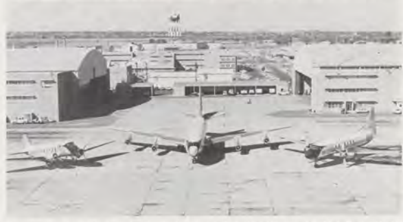
These are the "birds" that check accuracy of air navigation aids. The venerable DC-3 is at left. The C-135 (center) operates above 20,000 feet; The Convair 440 (r.), performs between 10,000 and 20,000 feet.
