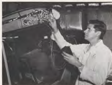
Joseph Fitzgerald, Gills Aircraft Service in Anchorage, makes voltmeter check; one of many maintenance types required of aircraft mechanics.
