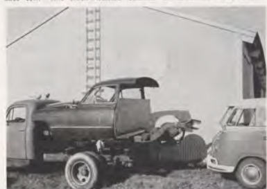
Other ways of launching a sailplane besides the aero tow include auto tow. This truck-mounted Cadillac is nicknamed "The Beast."
