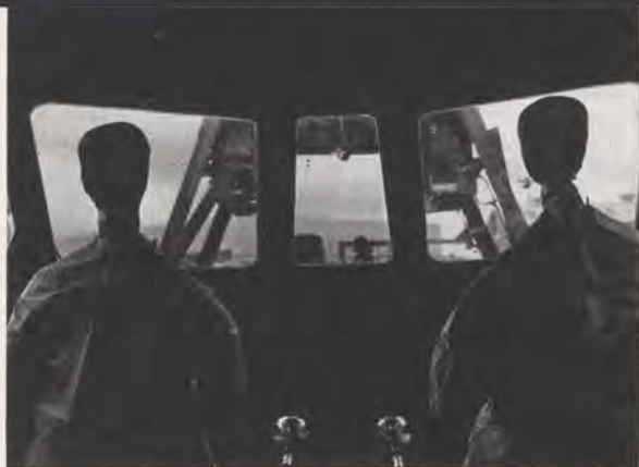
To simulate actual flying conditions, this photograph demonstrates how life-size pilot and co-pilot dummy men are placed in normal positions inside the cockpit area of the fuselage during a "bird impact test."
