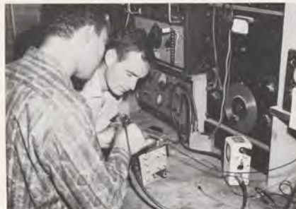
Electronic Equipment Maker and Repairer Donald Kenny (left) repairs a Transceiver with Arthur Bowen. The Fabrication and Laboratory Shop repair operation facilitates near-immediate reuse of items not in use because of breakdown.
