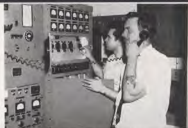
At LaGuardia Airport, John Lupack, electronics technician (left), briefs his chief, Herbert Pelton, SMS-35, during a check-out of the glide slope monitoring system which enables aircraft to assume the proper runway approach angle during landings. Safety is their big job.
