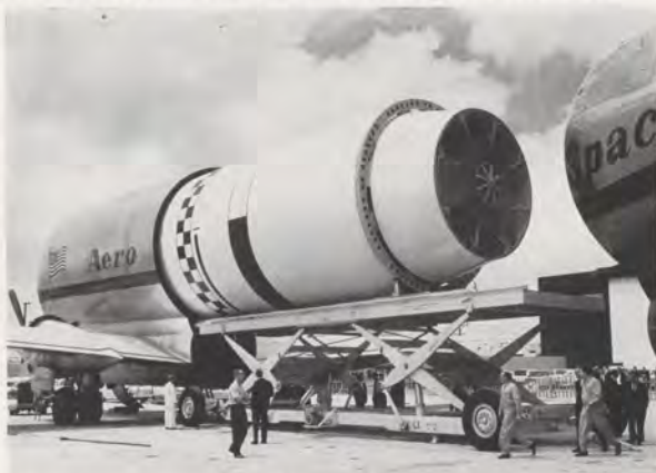
The "Pregnant Guppy" being assembled at FAA Hangar in Los Angeles before flight test with a dummy rocket.
