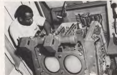
LaGuardia Airport electronics technician David Powell, SMS-35 (above), adjusts Precision Approach Radar. PAR-2 is "pulled" for on-the-spot adjustment. C. Sabela, Electronic Maintenance Section Chief (below), tests connections with E. Simon, Chief, SMS-33, NY International.
