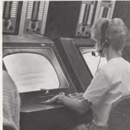
This display console (actually a closed circuit TV) permits operator to process flight plan information into a computer. In proper engineer language it is a component of Computer Driven Simulation Equipment, or briefly, CDSE.
