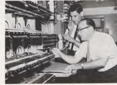
LaGuardia Airport electronics technician David Powell, SMS-35 (above), adjusts Precision Approach Radar. PAR-2 is "pulled" for on-the-spot adjustment. C. Sabela, Electronic Maintenance Section Chief (below), tests connections with E. Simon, Chief, SMS-33, NY International.
