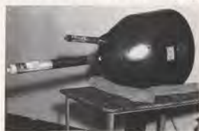
Two-gun charactron tube displays raw and processed video. Unique tube offers new possibilities.
