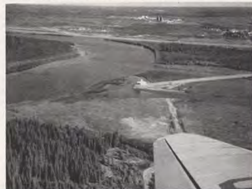
Concrete dike at Galena damaged by water and ice chunks 25 feet wide and 40 feet thick. Below, aerial view of VORTAC and site undermined by flood as new channel eliminates roadbed.
