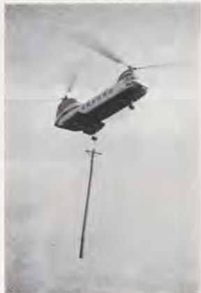
New York Airways helicopter is pulling a 30-foot external sling during a test flight at LaGuardia. This type of sling installation has been approved.
