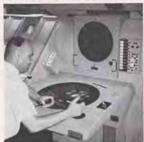
Stewart Morris, Air Traffic Coordinator, is shown seated at one of the RBDE-5 consoles. At the rear of the horizontal display, commonly called a "flatface," note the sector monitor which is used to complement the information presented on the flatface. Morris has "joystick" used in target identification in right hand.
