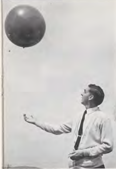
Goldee Boozer releases balloon. Timing its ascent by stop watch will enable him to compute ceiling level.
