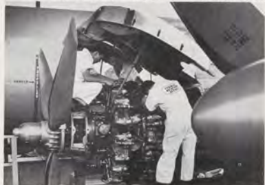
Checking the high tension ignition system coils in a Wright engine.
