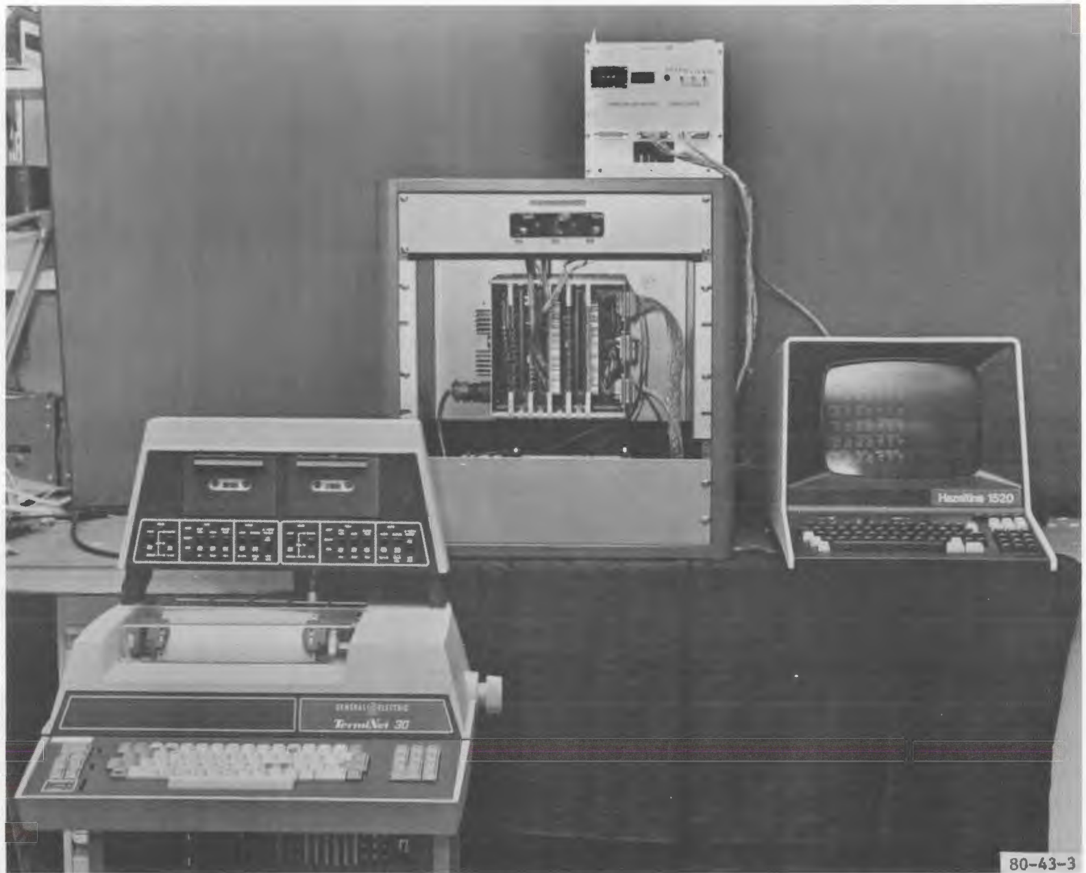
FIGURE 3. MICROCOMPUTER SDC, LED BAR-GRAPH DISPLAY, LOCAL MAINTENANCE TERMINAL, AND CASSETTE STORAGE UNIT
