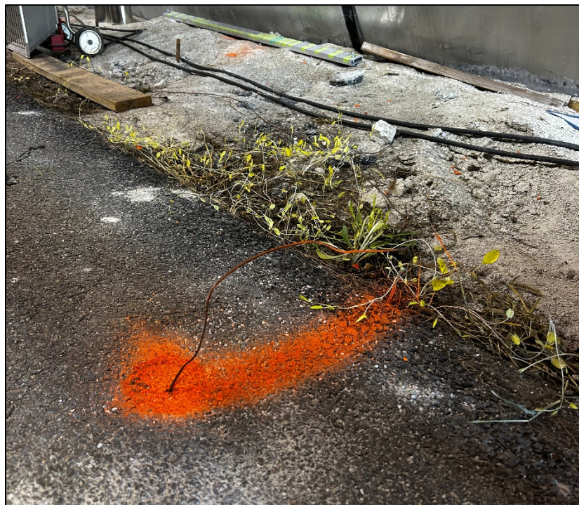
Figure 57. Photo. Verification thermocouple at section D4-50-12.5-0.
