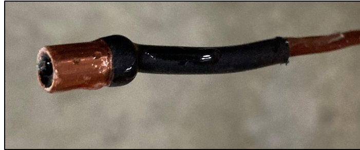
Figure 54. Photo. Finished thermocouple tip.
