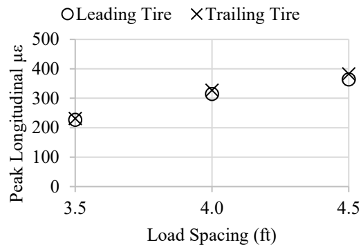
Figure 90. Graph. Effect of temperature and axle spacing on pavement responses in T1-80-12.5-0.
