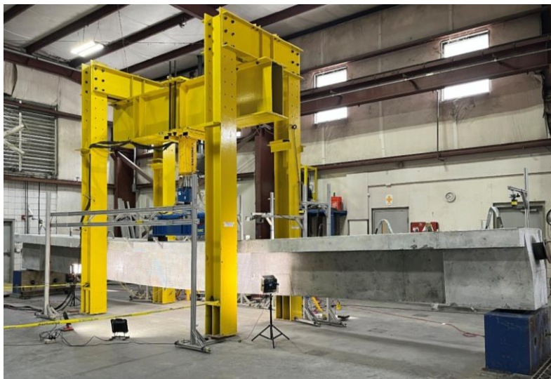
Figure 9.19. Flexural testing of the D19-P-T test beam.
