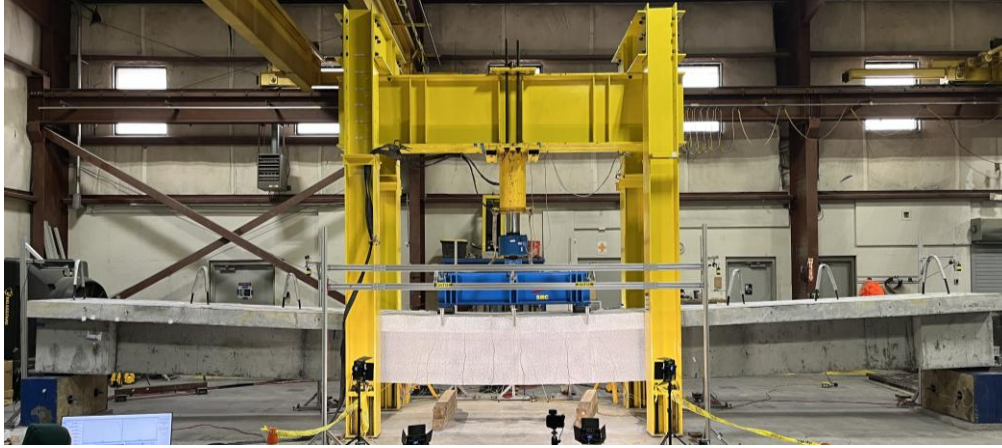
Figure 9.11. Flexural testing of S19-M-T test beam.
