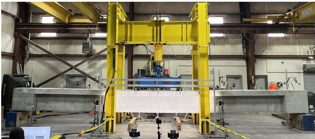
Figure 9.7. Flexural testing of S12-P-T beam
