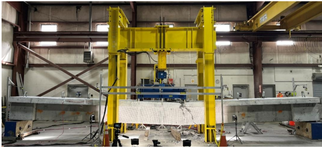
Figure 9.15. Failure of D19-M-U beam by crushing of top flange.
