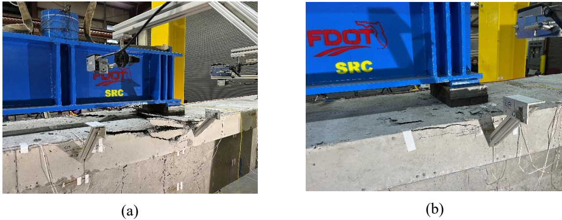
Figure 9.8. Crushing of concrete at the compression flange: (a) S12-P-U; (b) S12-P-T
