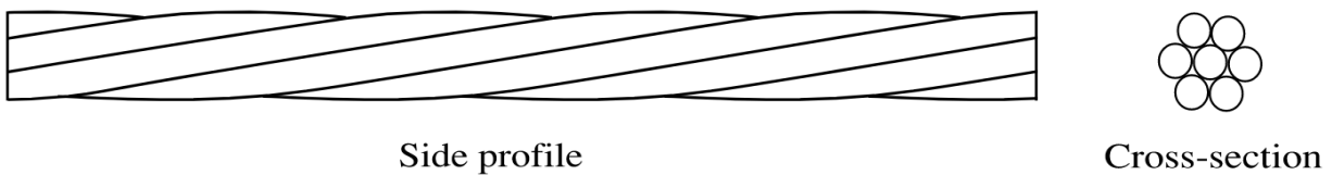
Figure 3.1. Seven-wire prestressing strand surface profile.
