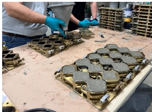
Figure 7.4. Pouring grout mix into cube molds.
