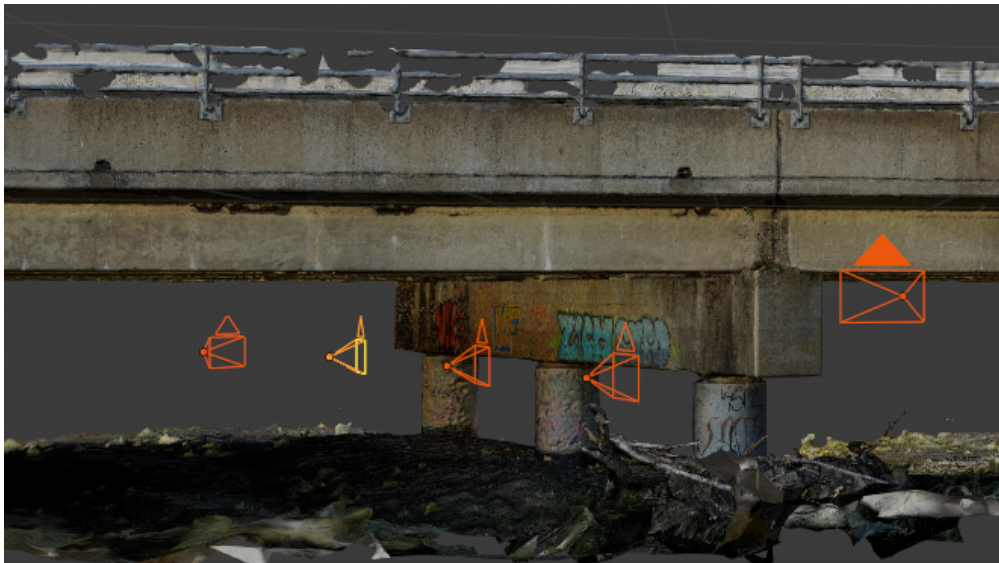
Figure 2.5: Planned viewpoints for Bridge 1 (20 0019Y) flight experiment (originally presented in the Task 4 report).
