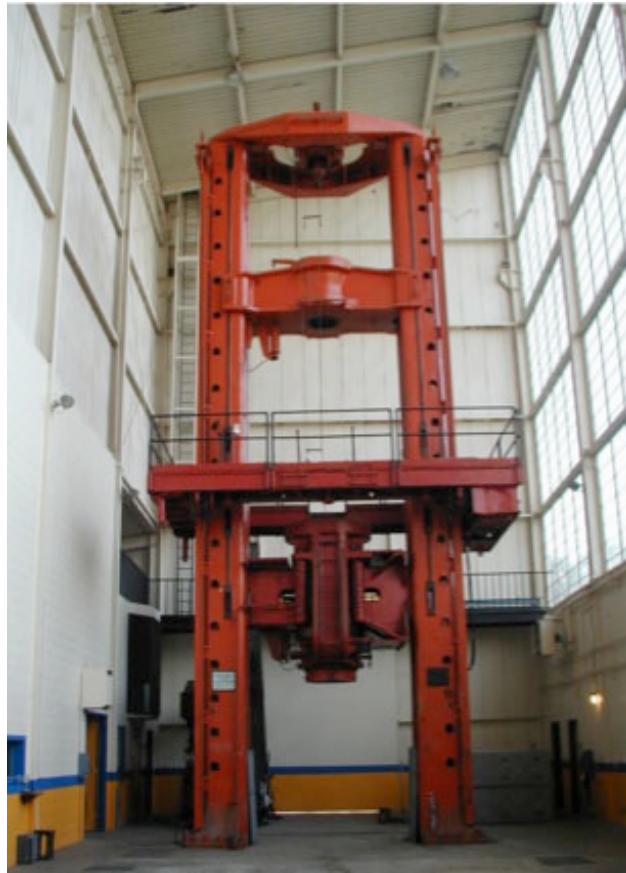
Figure 2.2: Big Press at PEER facility (originally presented in Task 3 report).
