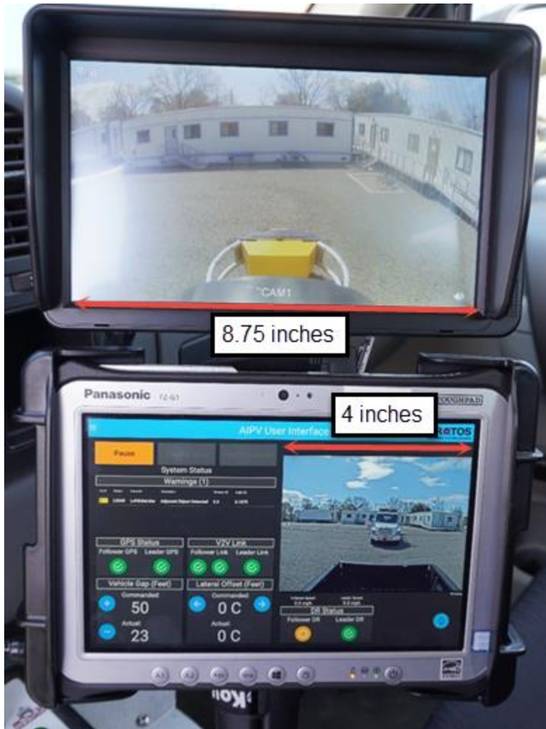
Figure 2.3: GUI in the LV with original camera view of the ITMA system
