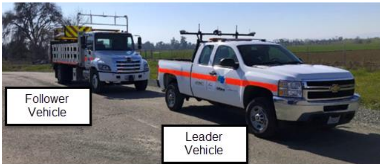
Figure 1.2: ITMA system defining the leader and follower vehicles
