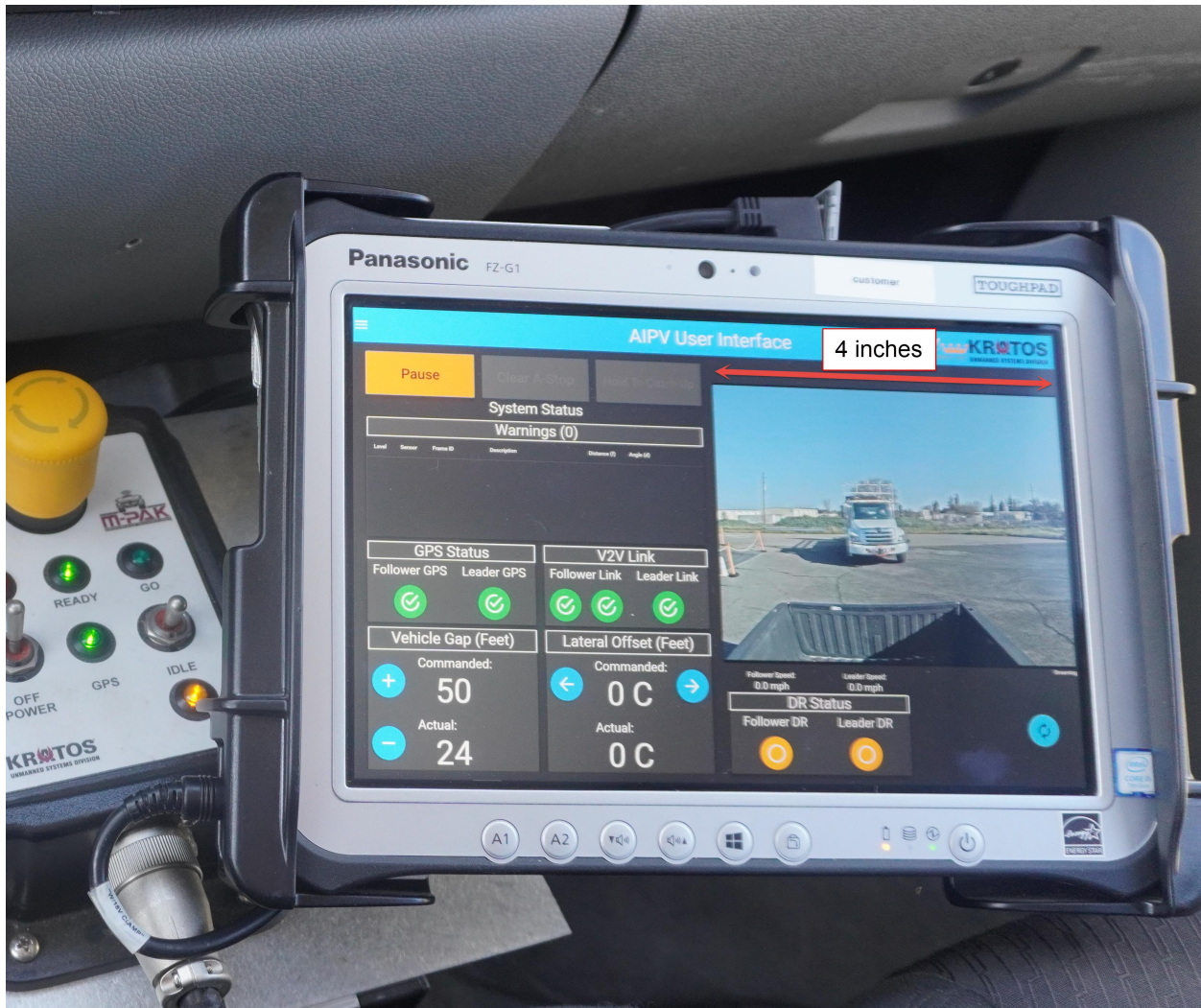
Figure 2.2: GUI in the LV with original camera view of the ITMA system
