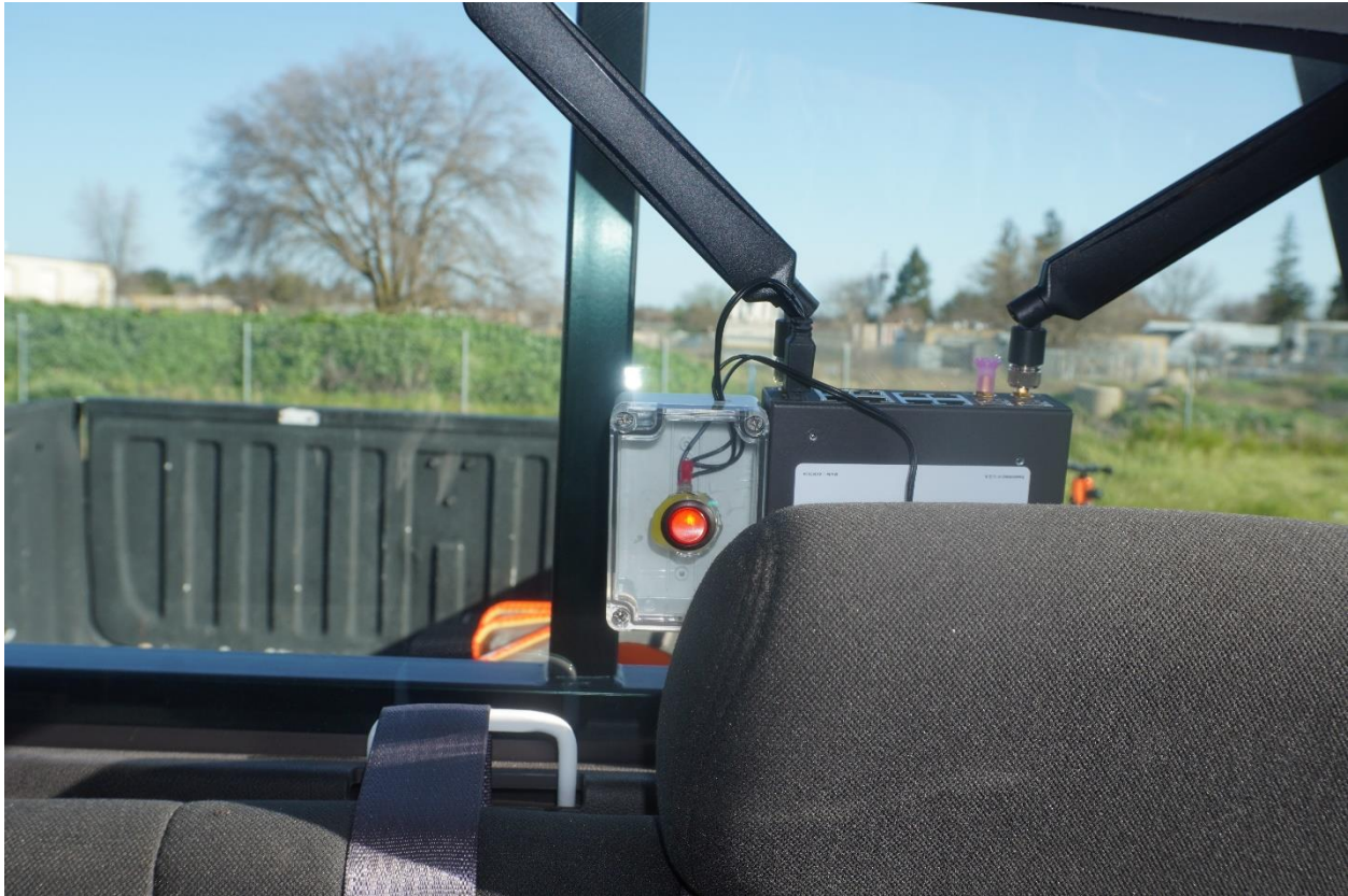
Figure 2.4: Cellular modem installed in the back of the LV for remote communication with the ITMA system
