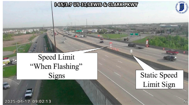
Figure 2.8 ITS Camera Image Along I-65 at MM 3.7 Showing a Variable Work Zone Speed Limit Trailer in Close Proximity to a Static Speed Limit Sign.
