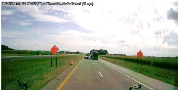
(c) "RIGHT LANE CLOSED AHEAD" Sign 2,500 ft in Advance of Merge Point
