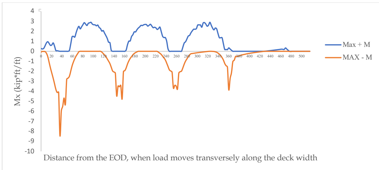
Figure 6.16. Moment envelope for deck slab with 9 ft girder spacing and two truck (Case 3.5)
