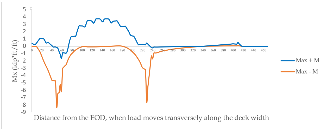
Figure 11.30. Moment envelope for deck slab with 15 ft girder spacing and single truck (with two cells)
