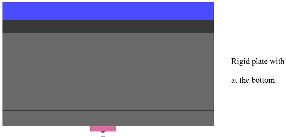
Figure 2.4. Rigid plate at the girder support with the applied boundary conditions
