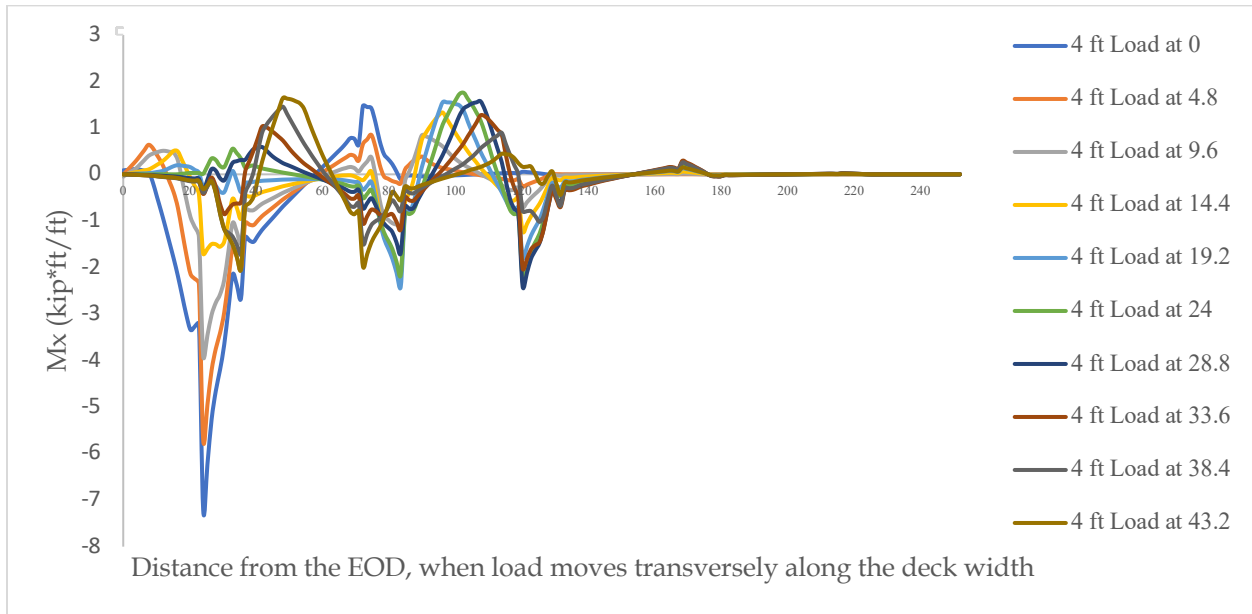
Figure 6.6. Moment diagrams for deck slab with 4 ft girder spacing and single truck
