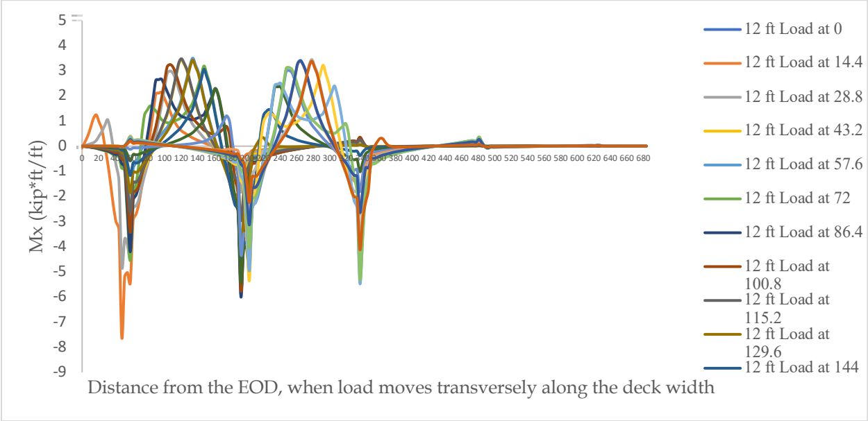
Figure 11.13. Moment profile for deck slab with 12 ft girder spacing and single truck
