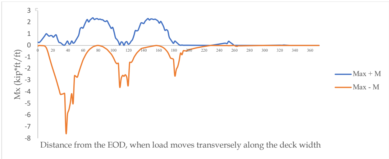
Figure 11.5. Moment envelope for deck slab with 6 ft girder spacing and single truck
