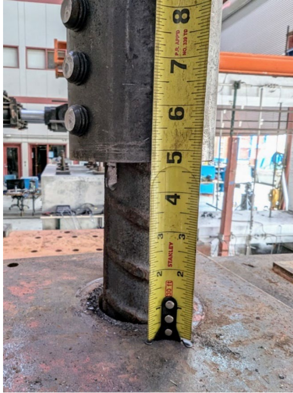
Figure 4.81: Residual displacement of bar grip at the end of the test
