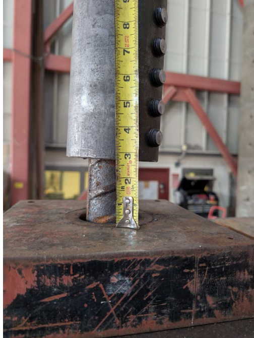
Figure 4.73: Residual displacement of coupler at the end of the test for Specimen 12
