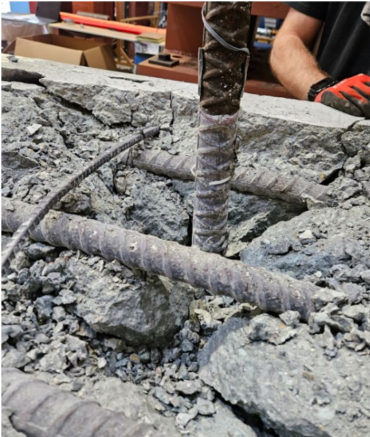
(b) Cone-shaped crack surface
