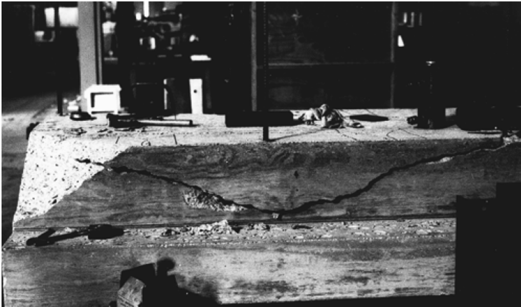
Figure 2.6: Concrete breakout failure in a shallow embedment test (De Vries et al. 1999)
