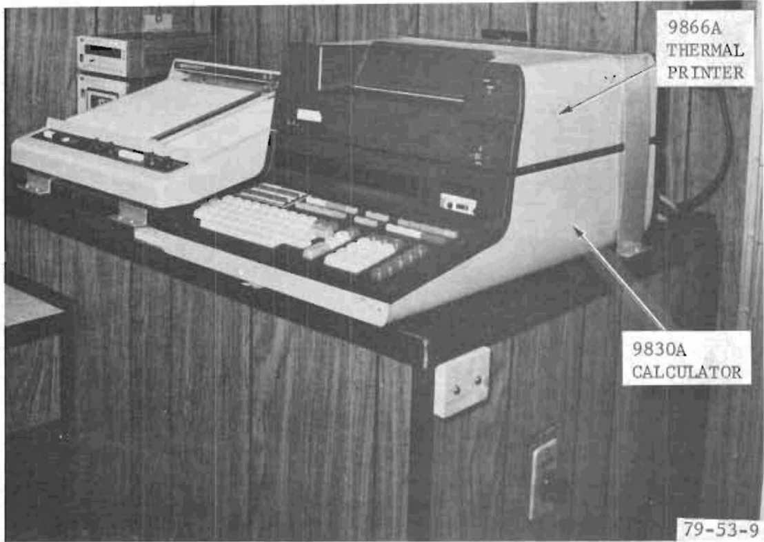
FIGURE D-4. PART OF MERF DATA ACQUISITION SYSTEM
