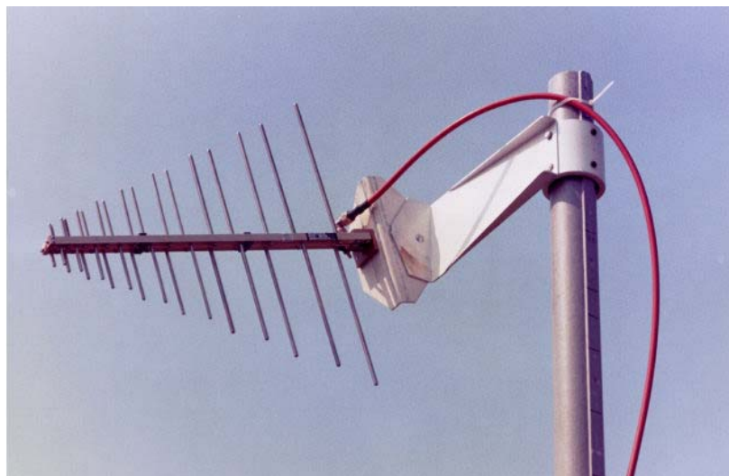
Figure 4: SAS-200/510 Antenna and Mounting Bracket
