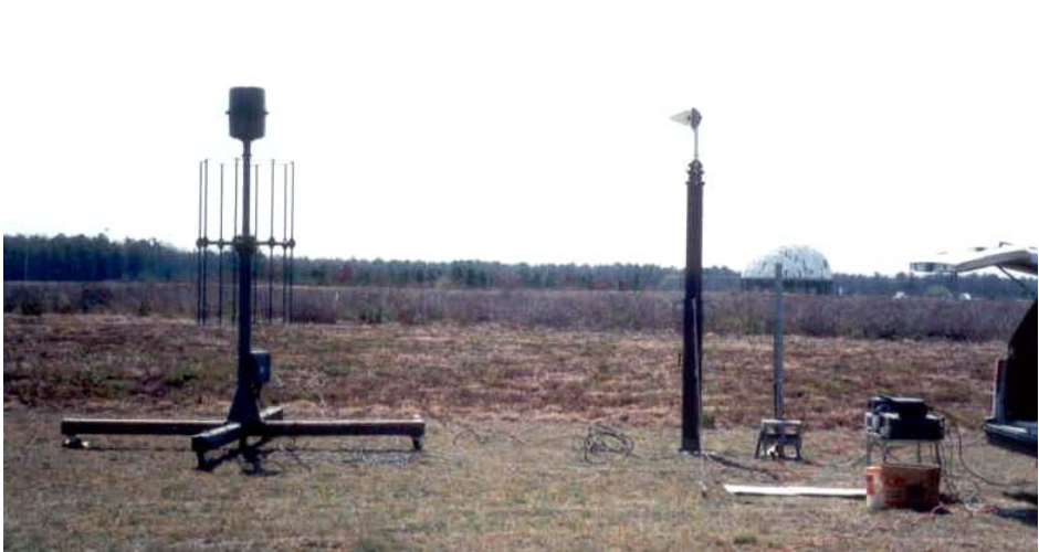
Figure 19: L-Band Interfering Antenna at 11.3 feet (boresite)
