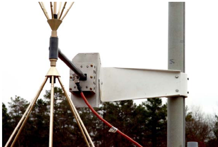
Figure 6: Biconical Mounting Bracket for Adaptation to Fiberglass Mast
