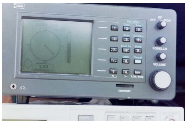
Figure 17: Bearing Displayed on DF Processor
