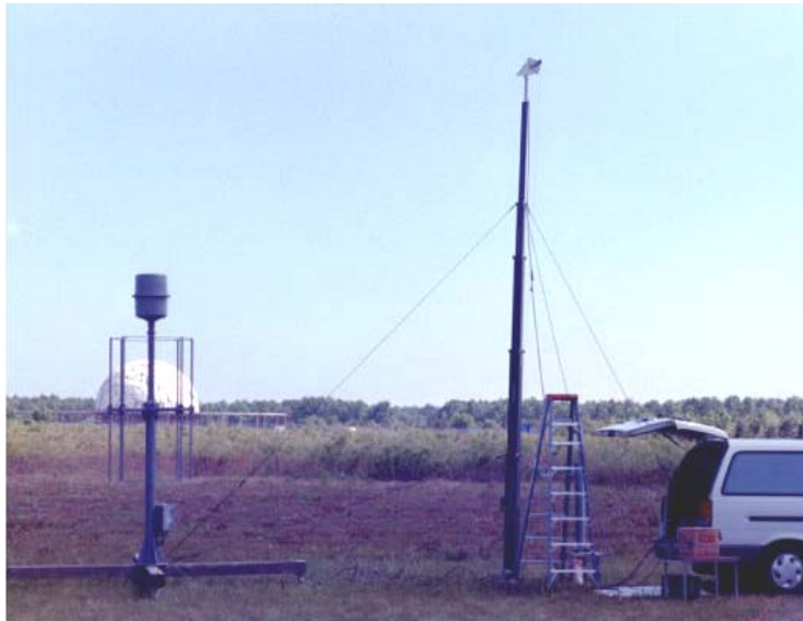
Figure 21: L-Band Interfering Antenna at 21 feet
