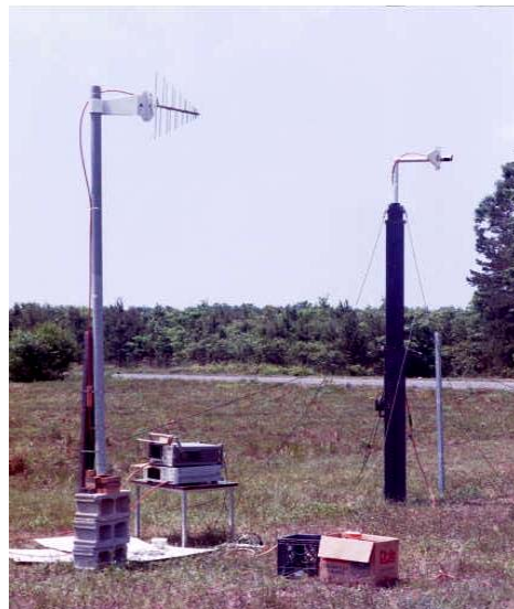
Figure 13: L-Band Field Strength Test Configuration
