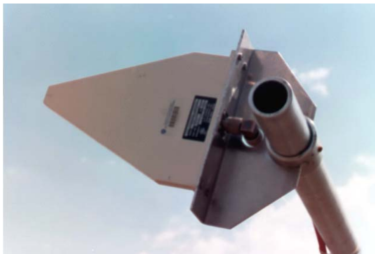
Figure 2: SAS-200/518 Antenna and Mounting Bracket
