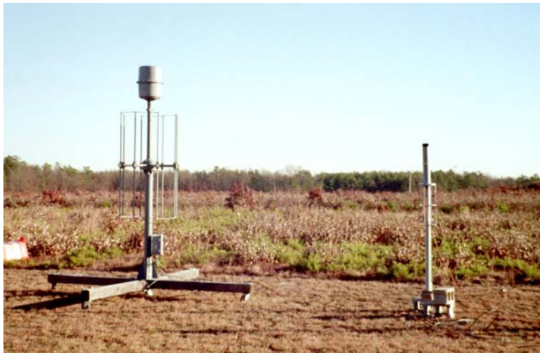
Figure 22: VHF-Band Interfering Antenna at 7.0 feet (boresite)
