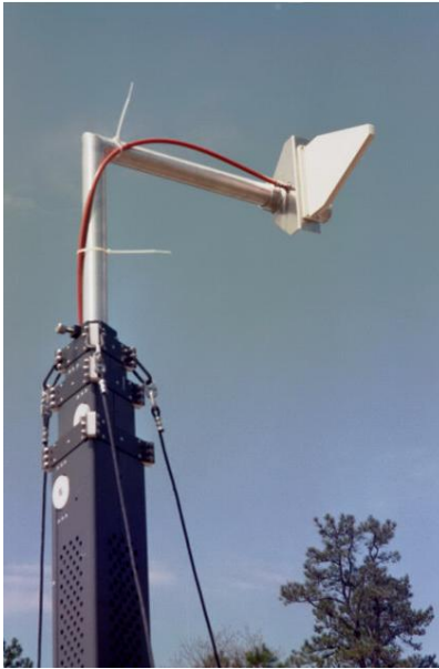
Figure 3: L-shaped Mounting Pipe for Adaptation to Military Mast
