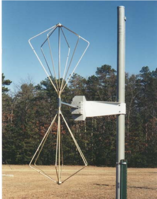
Figure 7: SAS-200/530 Biconical Antenna and Mounting Bracket
