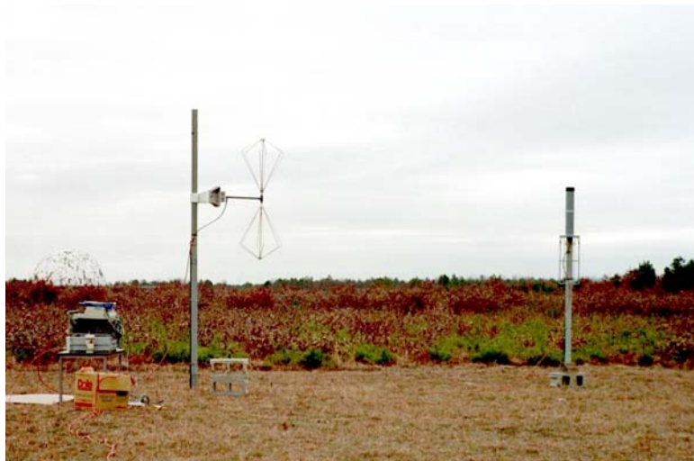
Figure 16: VHF-Band Field Strength Test Configuration
