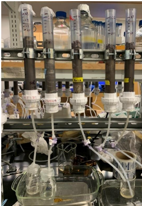
Figure 3.3. Experimental set-up for hydraulic conductivity test using the falling head method.
