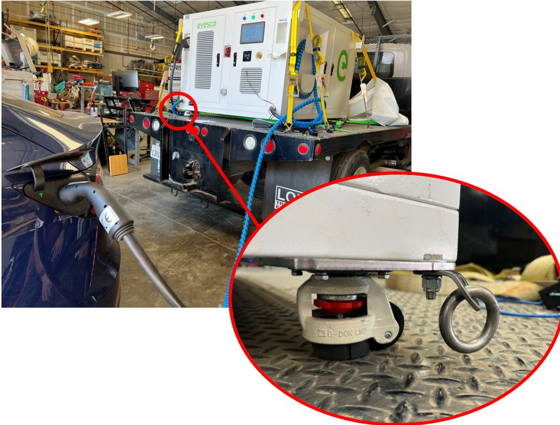
Figure 3.7: Mounting solution for attaching EVES-6060-NA to truck (including ratchet straps)
