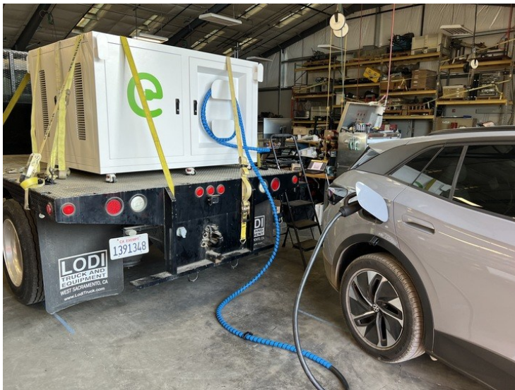
Figure 4.18: Volkswagen ID.4 being charged by the EVES-6060-NA
