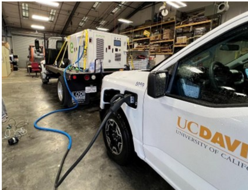
Figure B.16: Connecting the EVES-6060-NA charger to an EV
