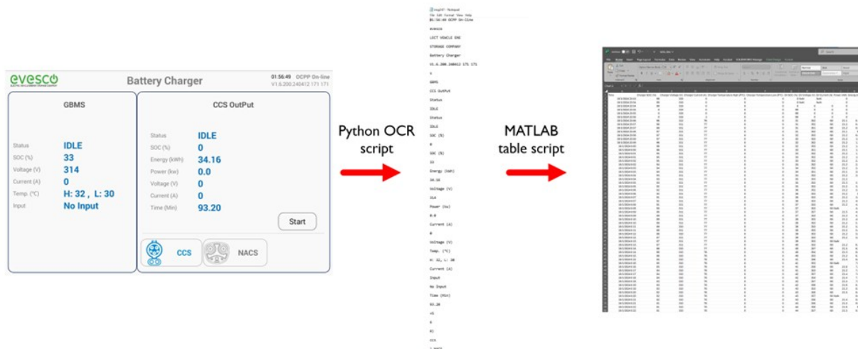
Figure 3.11: Flow of outputs from scripts ending in data table in .csv format
