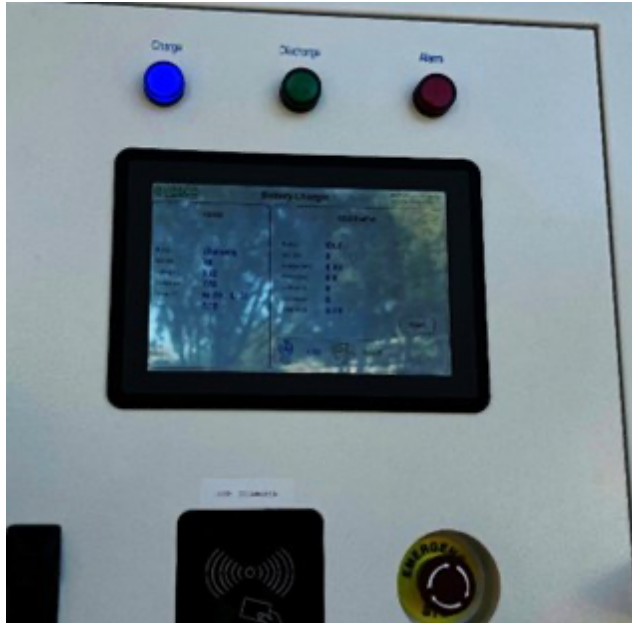
Figure B.12: Charging status display and indicator lights during AC charging operation
