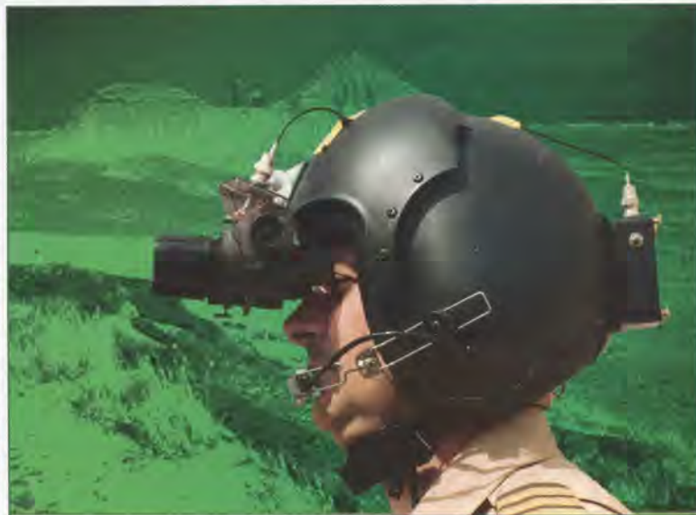
The background for this profile of the Helicopter Night Vision Device depicts the image the operator sees in the device. (The pilot's photo is by EG & G, the background by FAA's CAMI, and the digital montage by Mario Toscano.)
