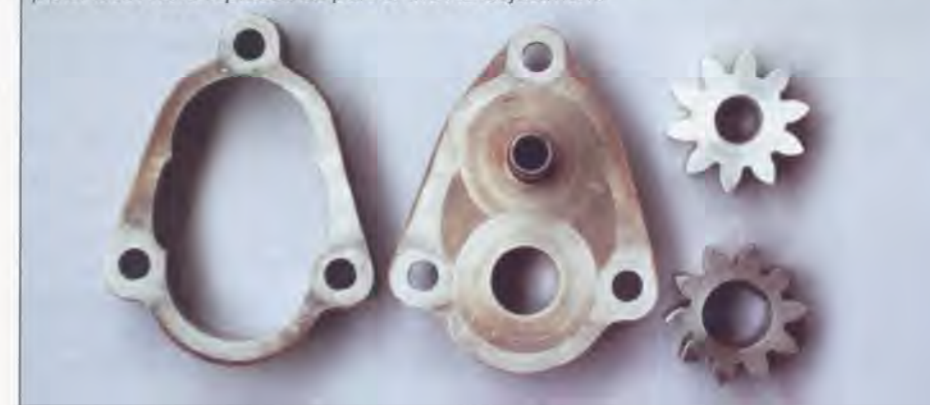
A most expensive paper weight. The aluminum oil pump impeller and its steel drive impeller both were replaced as part of the AD adjustment.
