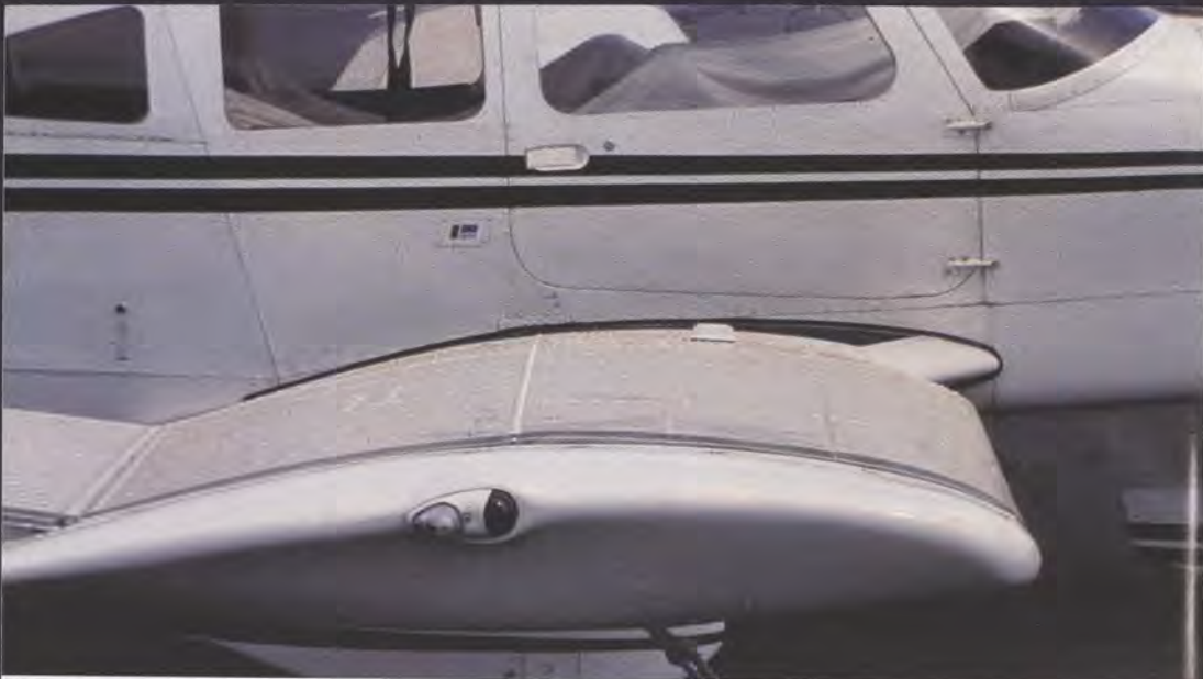
Check the wing top and bottom for bulges, cracks, and hangar rash.
