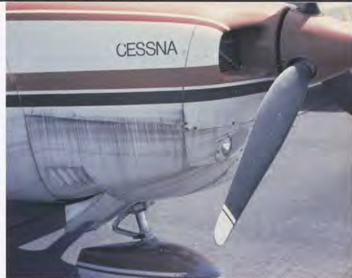
Check the paint stripes alignment before you measure spinner to cowling gap.
