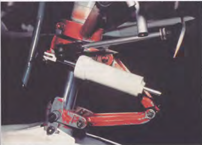
Shimmy dampers are designed to stop nose wheel shimmy, not cause it.
