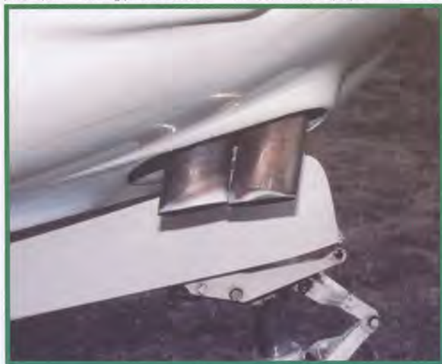
Dual exhaust pipes should never touch.
