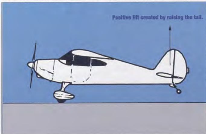
Figure 2 • Positive lift created by raising the tail for accelerating on departure roll.
