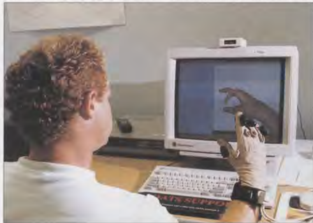
The glove used to sense hand position for virtual reality experiments. The hand on the CRT screen is computer generated and responds to the movements of the glove. This allows the operator to open the virtual drawers and move the virtual desktops. (FAA photo)
