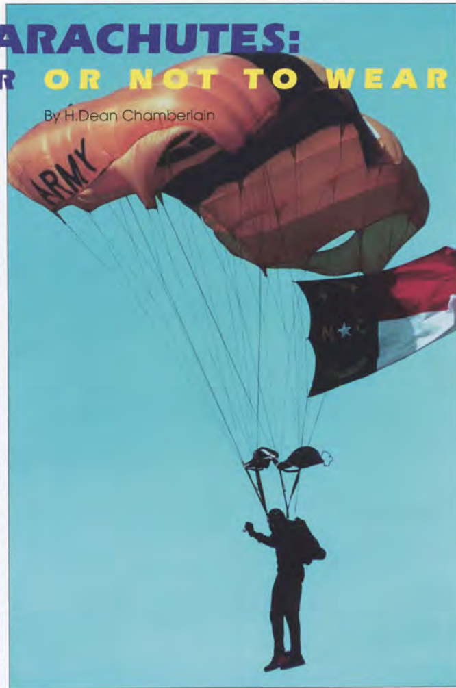
Ram-air style parachute canopies provide great maneuverability. Although used primarily by sport skydivers, such as this one being "flown" by a member of the U.S. Army Parachute Team, the Golden Knights, ram-air style parachute canopies can be custom ordered in some emergency parachute rigs. (AFIS photo)
