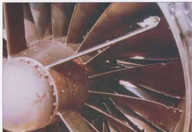
A close up of an engine damaged by Canada geese. (R. Dolbeer photo)
