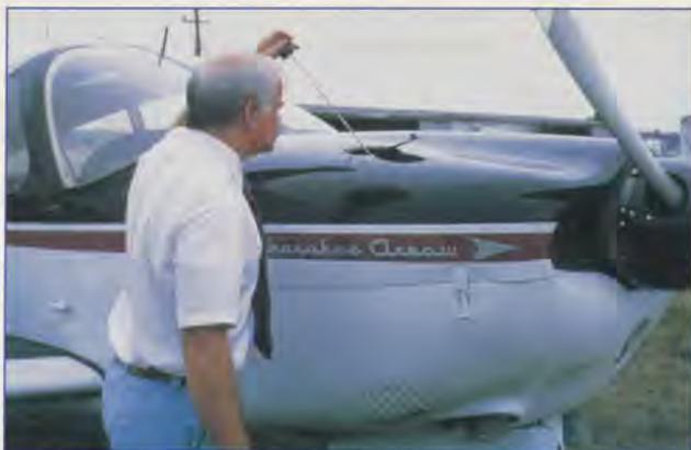
Oil is as important to the engine as fuel. Make sure the oil level and coloration are correct for your aircraft.
