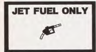
Many aircraft display decals next to their fueling port to eliminate the question of which fuel to use. All the line person has to do is match the color and legend with the design on the fuel pumps and nozzles. (See examples above.)
