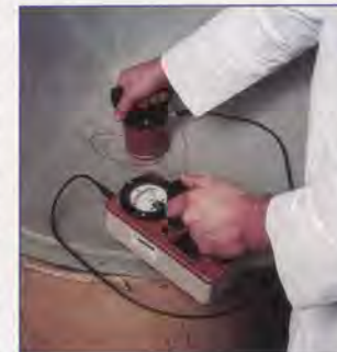
A technician scans a radome with a moisture meter to determine if moisture is present in the radome. Moisture scanning is a primary and simple trouble-shooting step, but radomes finished with antistatic coatings must be checked from the inside for accurate readings.
