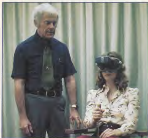
The Barony chair or "spatial spinner" demonstration helps pilots gain an understanding of how disorientation is induced and how to avoid it.
