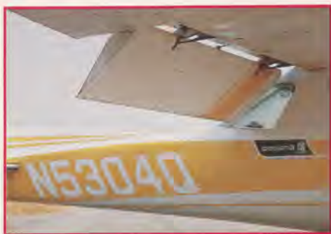
Figure 3. Located on the inboard portion of the wing of this Cessna 150 is a single slot Fowler-type flap. Airplane courtesy of the Professional Flight Service, Ft. Washington, MD.
