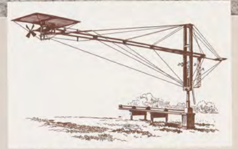
In 1891 Maxim built this machine for testing the efficiency of the screw-propeller and the lifting power of his airplane design.
