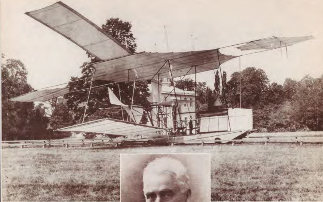
The crewmembers of Maxim's "aerial steamship" ready it for its trial run on its dual rail tracks. The craft had a 108-foot wingspan with twin 18-foot steam driven pusher propellers and a gross weight of 8,000 pounds. (The first successful Wright Flyer in 1903 weighed only 605 pounds.)
