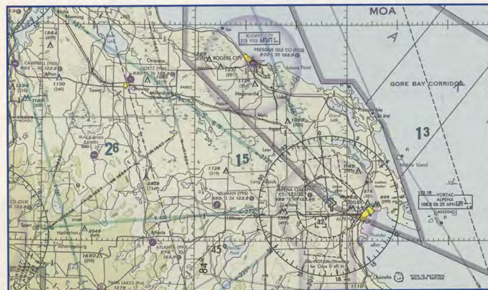
Look familiar? Above is a portion of the Lake Huron sectional chart with the old symbology for the control zone at Alpena. As of October 15, that same portion of the chart (below) will have a different look. The new symbology tells you that it is a control zone with a tower and arrival extensions without communications requirements. (NOT TO BE USED FOR NAVIGATIONAL PURPOSES.)
