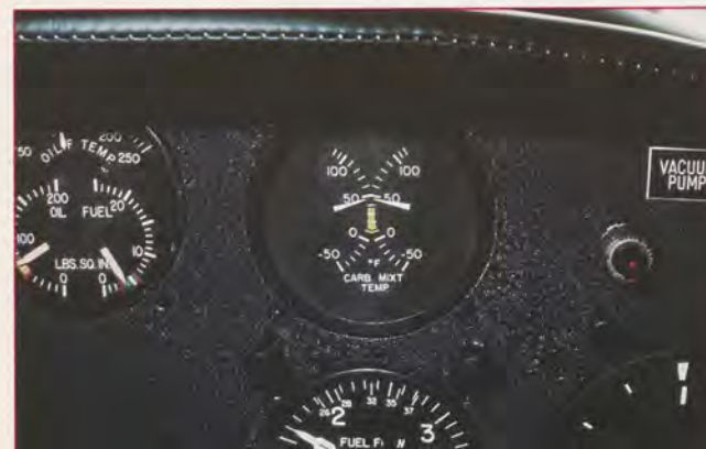
When the carburetor air temperature gauge needle is in the yellow arc, carburetor icing is most likely to occur.
