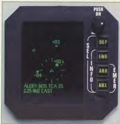
Figure 2. Data Link can provide real-time collision avoidance information for general aviation, using modifications to existing LORAN equipment.
