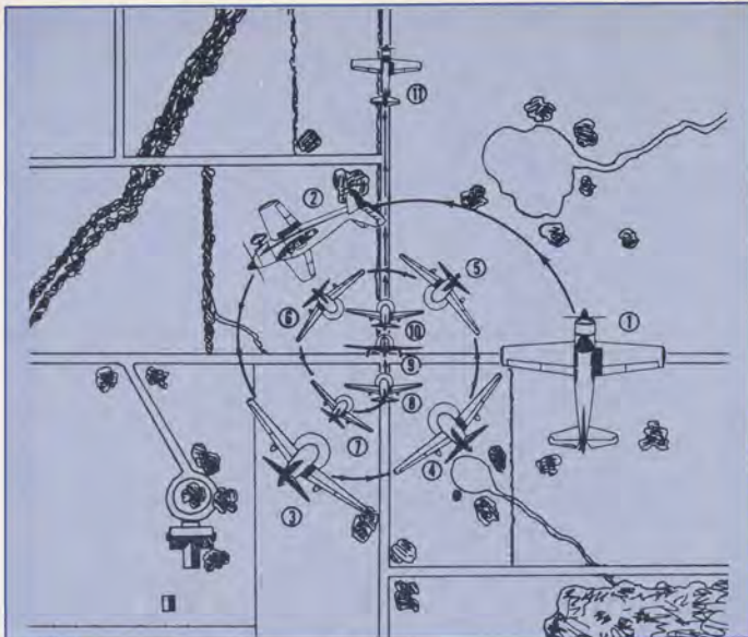
Figure 1. The first two turns of a spin and recovery (incipient spin) as seen from above. (1) Clear the area, line the airplane up with the road, and reduce power. Raise the nose to stall attitude and, as the stall approaches, use left rudder and full up elevator. Some airplanes may require the opposite aileron at the entry; others may need a burst of power (then reduced to idle) at this point. (2) The airplane is in the transient condition; some airplanes may move over to a slightly inverted position during this phase. (3) The spin is developing. (4) Hold the rudder and elevators in the fully deflected position. (5) Note that the path of the airplane is quite different from the spiral in that the airplane is flying a helix angle and is also rolling and yawing about its center of gravity. (6) Start recovery here or at (7), depending upon the airplane used. (8) The opposite rudder and forward motion of the control wheel starts to "bite." (9) Rotation stops, and the angle of attack is back in the flying range. (10) The pull-out is started. (11) The airplane returns to straight and level cruising flight. Be sure that the recovery is complete at least 2,500 feet above the surface.
