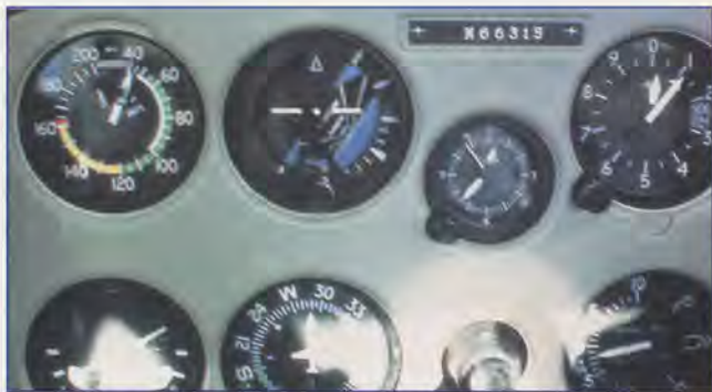
Instruments tell the story: Airspeed at stall, altimeter winding down in this spin to the left. Note that the attitude indicator has tumbled and does not give an accurate picture of the direction of the spin—use the bank indicator on the turn coordinator.
