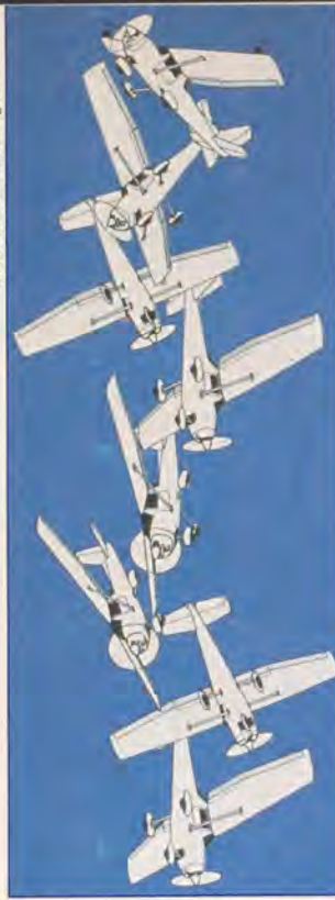
This illustration cannot do the rapidly developing spin rotation justice, but this is what it might look like in slow motion. Fast or slow, this situation is to be avoided.
