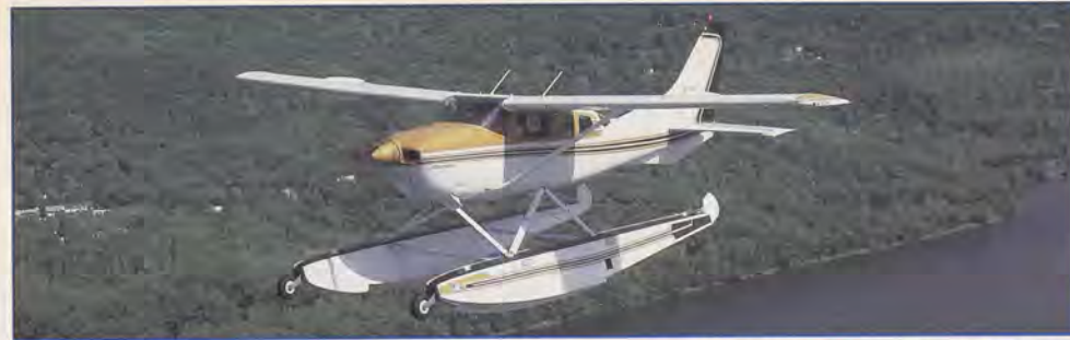
Addition of floats changes flight characteristics very little. The greater part of seaplane pilot training involves learning to handle the airplane on the water. In windy conditions you can even "sail" a seaplane.
