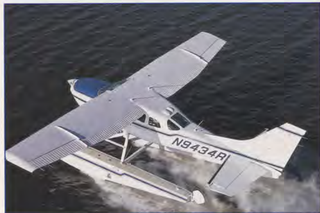
At application of takeoff power, the seaplane begins to plough taxi until it gets up "on the step" where the plane can accelerate while just barely on the surface of the water.
