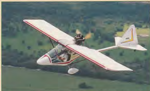
Is it an airplane or an ultralight? In this case it is an ultralight registered as an experimental aircraft.
