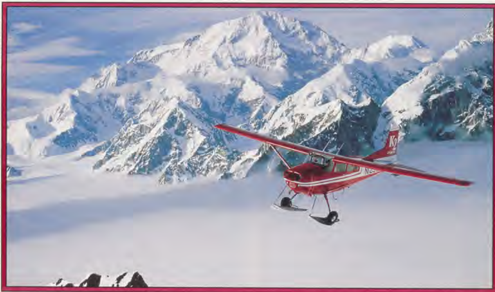
Denali, a mountain between Fairbanks and Anchorage in the Alaska Range, serves as a magnificent backdrop for a Cessna 185 on skis, a common winter landing gear in Canada and Alaska. Ground fog often obscures glacier landing sites on Denali, but Alaskan air taxis routinely land there and pass weather information on to others flying in the area.
