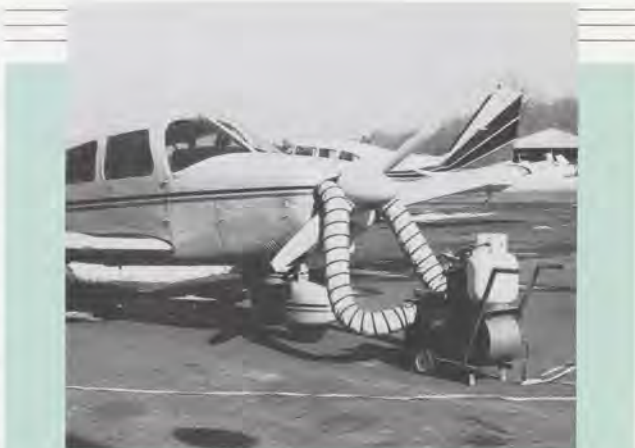
When preheating an engine, use only an approved aircraft preheater and follow the manufacturer's instructions. Remember to preheat the cockpit.
