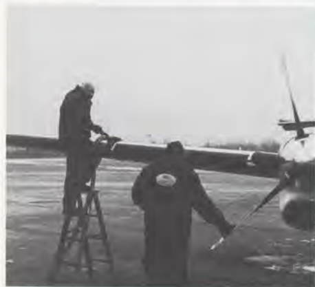
To avoid condensation in the fuel tanks, top them after each flight.
