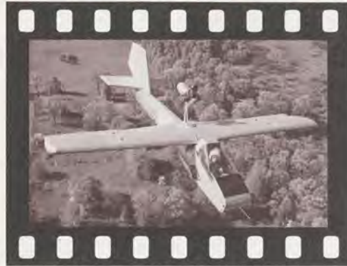
A unique inflatable aircraft developed by Goodyear Aerospace Corporation, proposed for use as an advanced military drone, a remotely piloted vehicle or an escape/rescue vehicle. The firm built and test flew 12 of the aircraft during the 1950s.
