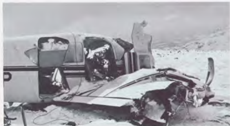
Severe structural damage can produce delayed ignition of fuel vapors from sparks given off by shorted electrical components or by broken power lines struck by aircraft. This Aztec twin crashed in the White Mountains of New Hampshire after striking high tension wires.
