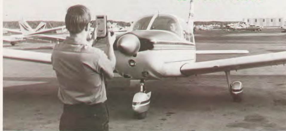
Mechanic dials in numbers on test instrument as he prepares to take reading from spinning prop, for comparison with airplane tachometer.
