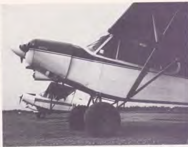
Use of oversized "tundra tires" on PA-11 constitutes major alteration, must be approved.
