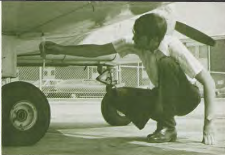
Your chances of getting all the water out of the tank will be better if you rock the wings gently before draining the sumps.
