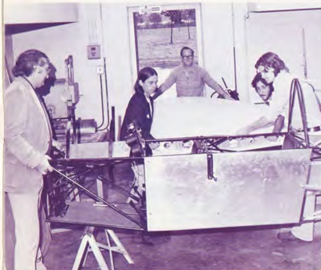
Wing is fitted to the Sonarar II by Lake Taylor students aided by EAA members Henry Proescher, left, and Dick Robbins at wingtip. Above, teachers and advisors pore over plans during an evening session at Lake Taylor.
