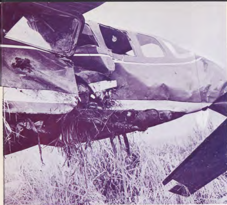
Above—the force with which the aircraft impacted the ground was clearly evident when the crumpled Skywagon was hoisted from the accident site during the investigation. Left—Goroka Airdrome, in north Australia showing flight path and scene of the crash. Photos courtesy of Aviation Safety Digest.
