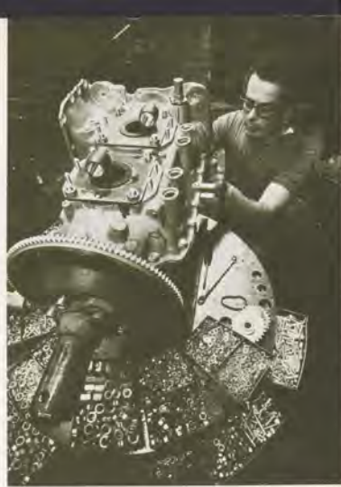
Four-cylinder Lycoming engine, in for remanufacture, is disassembling for inspection and replacement or repair of all worn parts.
