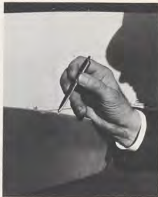
Left—good pre-flight propeller inspection includes looking for grease or oil leaks and feeling for looseness, damage, cracks and nicks. Above—the leading edge is most vulnerable to prop nicks and their effects.
