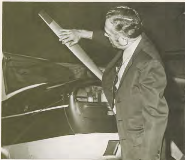
Left—good pre-flight propeller inspection includes looking for grease or oil leaks and feeling for looseness, damage, cracks and nicks. Above—the leading edge is most vulnerable to prop nicks and their effects.
