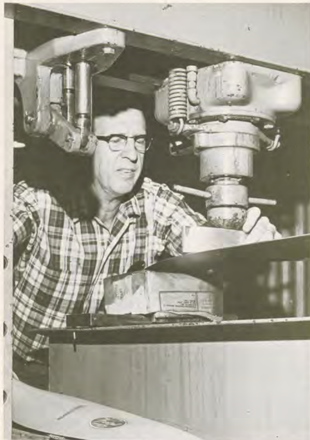
Some types of bends in prop blades can be straightened, as above, on a hydraulic press.
