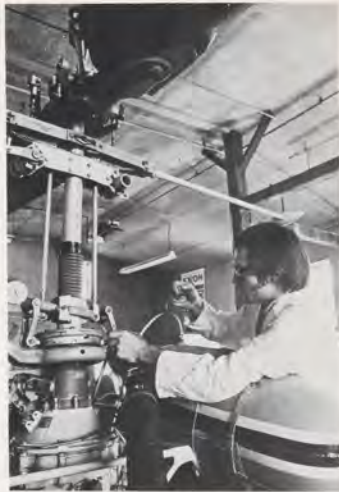
The rotor mast is "nerve center" of the helicopter's flight mechanism. The security of every bolt is vital to safety. Here mechanic Kevin Martin inspects the swash plate.
