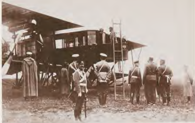
Four 100 hp engines lifted this five-ton pre-World War I flying pleasure carriage, Le Grand , into the air successfully. Right—Igor Sikorsky, pioneering genius of large-scale aircraft.
