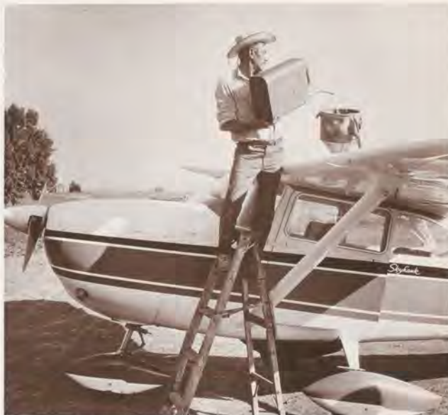
If you have never fueled by hand, learn how it is done properly. Filtering and grounding are essential, and should be carried out or personally overseen by the pilot.
