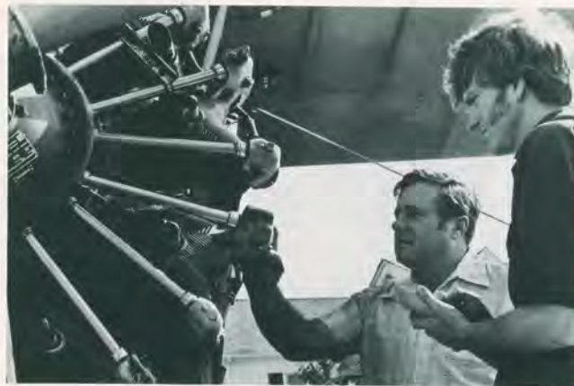
Johnson goes over maintenance check list with chief mechanic. Aircraft are washed down after each mission, to reduce corrosion.
