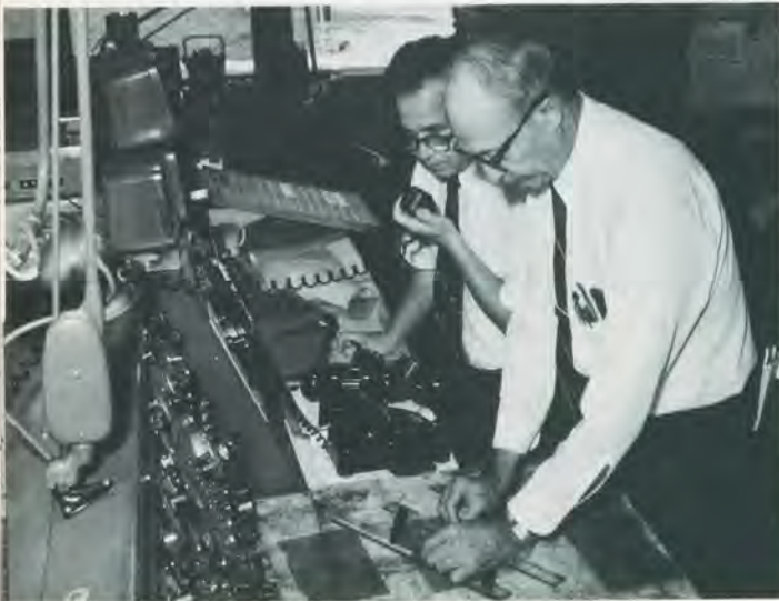
The DF bearing may be used in conjunction with VOR or other NAVAIDs to fix location of any aircraft in trouble. Ground observation, when possible, is also important.
