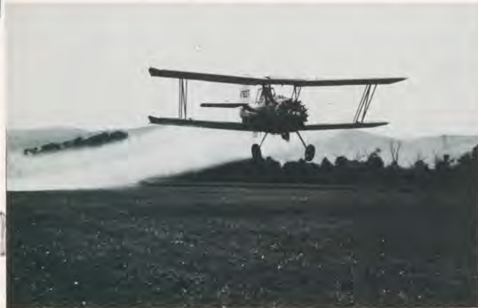
Laying it down on the ground where it ought to be. Dusting alfalfa near Magnolia, Del., in a 450 hp Ag Cat. The still morning air cuts down on drift, and possible crop contamination.
