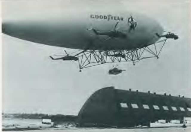
TANKS A LOT. The Helistat , proposed new vertical lift vehicle combining best features of helicopters and airships, is intended to lift and move payloads beyond the capability of current highway, rail and air transport systems. Three million cubic feet of helium add to the lift of the four Sikorsky helicopters. Scale model shows how 62-ton battle tank might be lifted.
