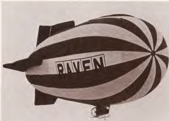
RETURN OF THE AIRSHIP. Presently undergoing tests in Sioux Falls, S.D., is the experimental Enterprise , first hot-air airship to be built in this country. Powered by a modified Revmaster VW engine, the craft is 120 feet long, 48 feet in diameter, carries a crew of two, and can travel from 5 to 25 miles per hour. Possible uses are traffic watch, crowd control, environmental observation (like checking oil spills), and advertising.
