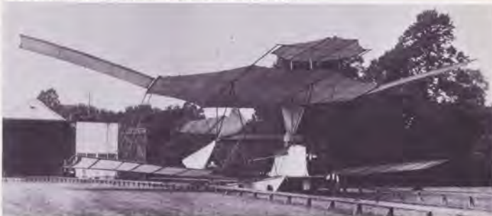
The 105-foot wingspan of Maxim's huge craft dwarfs crew members readying the "aerial steamship," with its twin 18-foot steam-driven pusher props, for a trial run on tracks.
