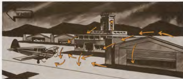
Above—on an otherwise smooth day winds blowing across hangars may result in turbulence over the runway. Below—approaching a mountain peak to leeward, aircraft may encounter unseen downdrafts several thousand feet above the crest, several miles from the mountain.
