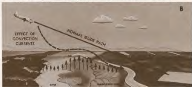
Depending on the surrounding terrain, convective currents—localized vertical air movements—can cause either overshoot (above) or undershoot (below) during landing.
