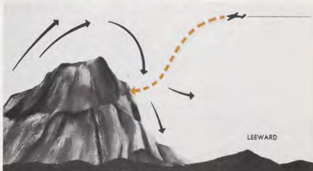
Above—on an otherwise smooth day winds blowing across hangars may result in turbulence over the runway. Below—approaching a mountain peak to leeward, aircraft may encounter unseen downdrafts several thousand feet above the crest, several miles from the mountain.
