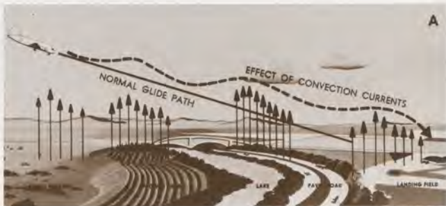
Depending on the surrounding terrain, convective currents—localized vertical air movements—can cause either overshoot (above) or undershoot (below) during landing.
