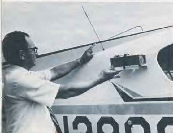
ELT permanently installed in Baron , above, sits on shelf just inside of point indicated by pilot. Interior view (upper right) shows attachment to outside antenna. Lower right—portable ELT sits in bracket firmly mounted on fuselage. Mounting on seatback is not advisable.
