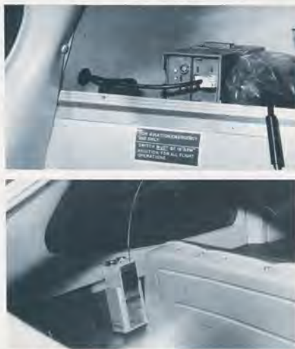
ELT permanently installed in Baron , above, sits on shelf just inside of point indicated by pilot. Interior view (upper right) shows attachment to outside antenna. Lower right—portable ELT sits in bracket firmly mounted on fuselage. Mounting on seatback is not advisable.
