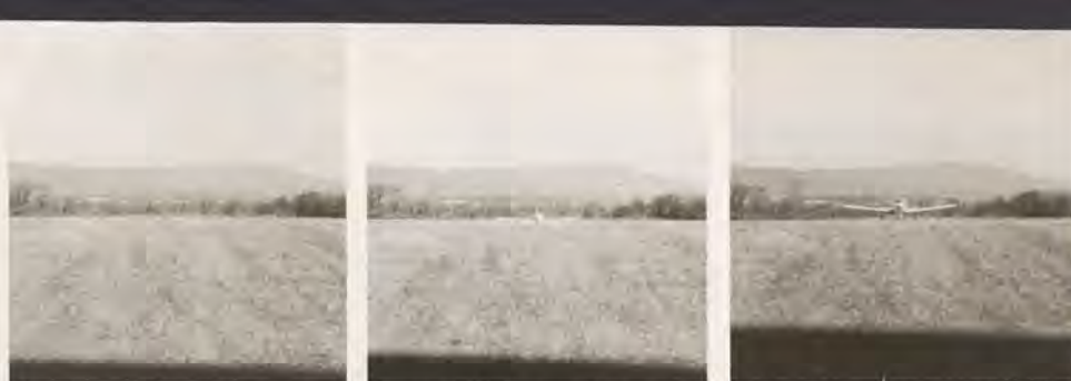
Watch closely: on an up-and-down-hill airstrip such as the one in the series of photos above, takeoff run is well under way before the airplane becomes visible from the opposite end of the field. With calm, variable, or crosswinds, both ends of the runway could be "active."
