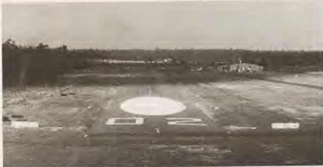
SHAPE OF THE OVAL on the runway tells the pilot whether he is on the proper approach path for landing, in this experimental visual aid. If the oval appears round, the plane is approaching at or near the proper angle; if elongated, it is high; if it appears flattened, the plane is low. Other designs being tried use a diamond, and a pair of rectangles. Tests were conducted at FAA National Aviation Facilities Experimental Center at Atlantic City.
