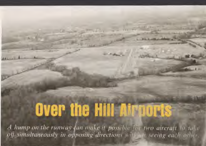
Watch closely: on an up-and-down-hill airstrip such as the one in the series of photos above, takeoff run is well under way before the airplane becomes visible from the opposite end of the field. With calm, variable, or crosswinds, both ends of the runway could be "active."
