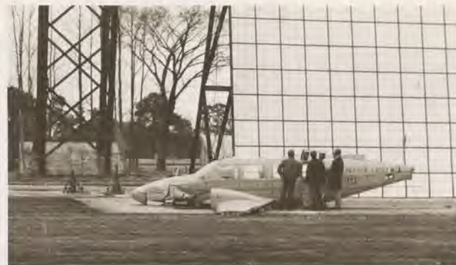
Left—actual aircraft, complete with instrumented dummy, being dropped from 350-foot tower in controlled crash during tests at Langley Research Center. Above—after the crash.
