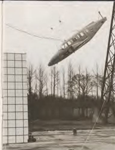
Left—actual aircraft, complete with instrumented dummy, being dropped from 350-foot tower in controlled crash during tests at Langley Research Center. Above—after the crash.
