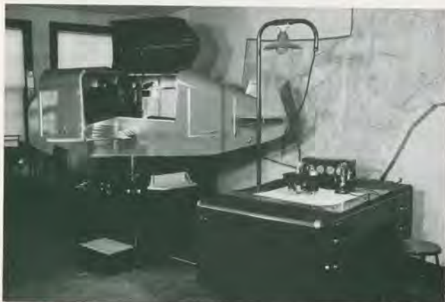
Above—This trainer records your progress. From the desk an instructor can radio instructions, then monitor instruments and flight path as it is drawn automatically on chart.
